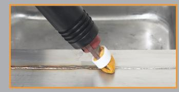
SURFOX is a safe, effective and fast electrochemical cleaning system. Passivation begins instantly after the SURFOX electrochemical cleaning process is completed. It usually takes between 24 to 48 hours for passivation to be stable and complete.
