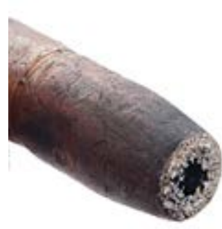
Nozzle fully clogged (not using E-WELD Nozzle)
